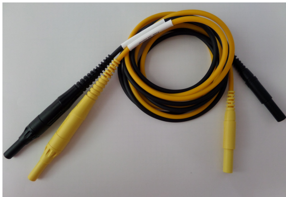
Figure 5.18: Fused safety laboratory leads for voltage path
