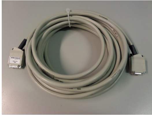
Figure 5.9: Shielded DSUB9 extension cable
