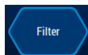
Figure 7.5: Soft key to trigger an action. In this example, the triggered action is to edit filter settings. When this soft key is pressed, a sub-menu is opened which allows users to configure the filter settings.
