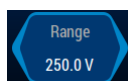
Figure 7.7: A disabled soft key which still displays a state. Although similar to the soft key in Figure 7.6 [→147], this soft key displays the current setting. This happens usually in conjunction with automatic functions. In this example, the auto-ranging mechanism is active, so it is not possible to manually change the range but the soft key provides information on which range was selected.
