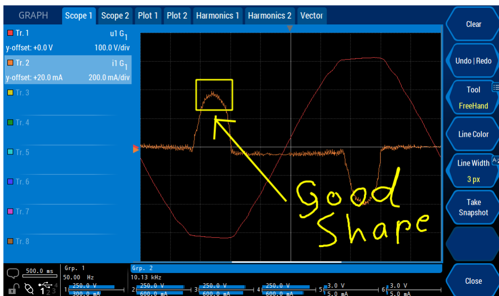
Figure 7.10: The on-screen painter. It can be opened in the on-screen menu (see ON-SCREEN MENU [7.1.1→149]).
