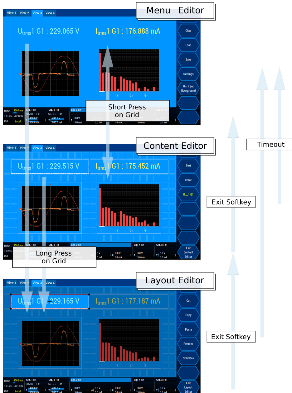
Figure 7.15: The different edit level of the custom menu.
