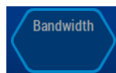
Figure 7.6: Soft key which is currently disabled as the key is not applicable in the current context. Pressing has no effect. Once the context is changed in such a way that this soft key has a purpose, the soft key will be activated again.
