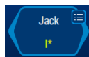
Figure 7.4: Soft key to change an entry from a list. The selected value of the list is displayed. By pressing either the left or right side of the soft key, the previous or next value of the list is chosen, respectively. In most cases, the selection will be wrapped-around to beginning once the end of the list is reached. A long press will open a selection dialog.
