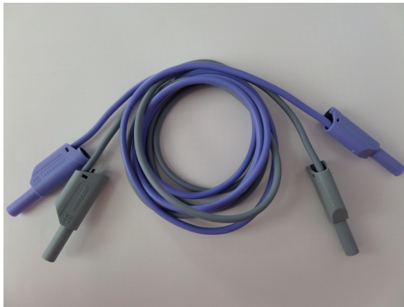
Figure 5.17: Safety laboratory leads for current path
