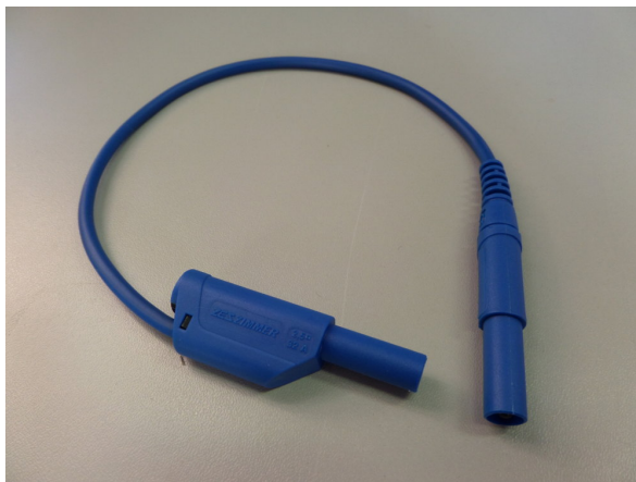
Figure 5.19: Safety laboratory lead for general purpose
