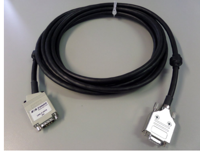
Figure 5.8: Shielded Sensor extension cable with extended temperature range
