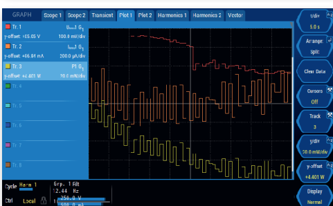
Display of measured RMS values
